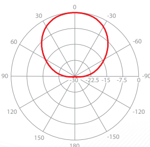
V/H - Port Pattern Elevation 5.6 GHz
