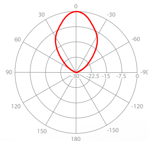
V/H - Port Pattern Elevation 5.6 GHz
