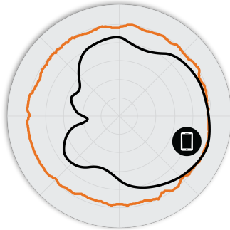
Figure 3. M510 5GHz Azimuth Antenna Patterns
