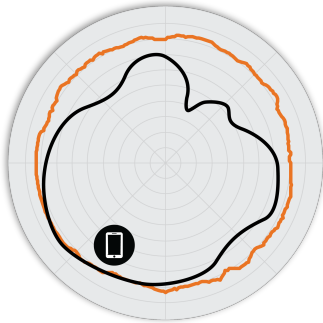
Figure 2. M510 2.4GHz Azimuth Antenna Patterns
