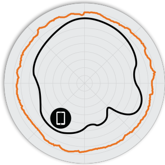
Figure 2. E510 2.4GHz Azimuth Antenna Patterns
