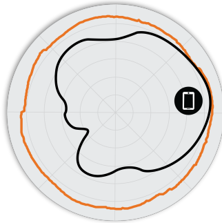
Figure 3. E510 5GHz Azimuth Antenna Patterns
