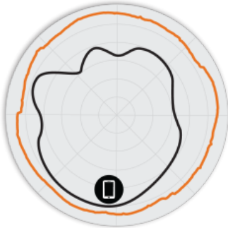
Figure 2. T811 2.4GHz Azimuth Antenna Patterns
