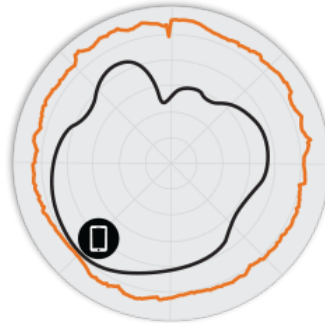
Figure 3. T811 5GHz Azimuth Antenna Patterns
