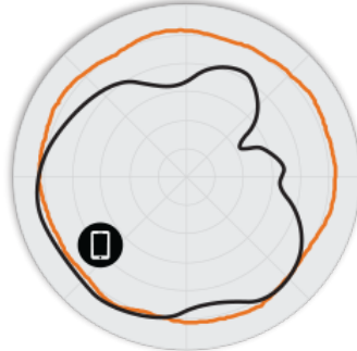
Figure 3. R610 5GHz Azimuth Antenna Patterns
