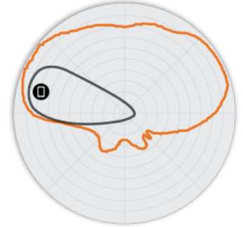
Figure 5. R610 5GHz Elevation Antenna Patterns
