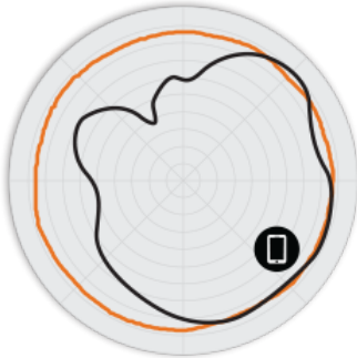
Figure 2. R610 2.4GHz Azimuth Antenna Patterns
